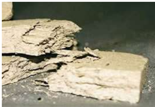
Pieces of Asbestos Insulating Board (AIB)
